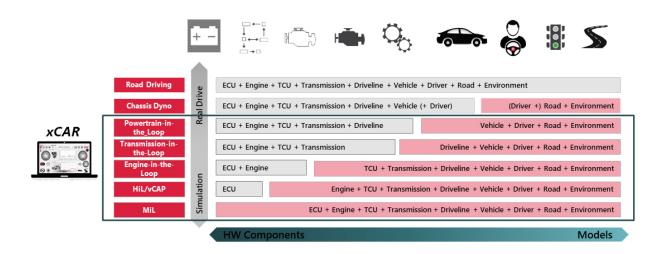
The xCAR™ XiL application offers a model structure describing the entire vehicle for any type of powertrain, with e.g. an engine block, a battery block, an electrical block, a vehicle block, a transmission block, an energy management system block and a driver block. The interface has been created to be used not only by simulation specialists but also by calibration engineers
